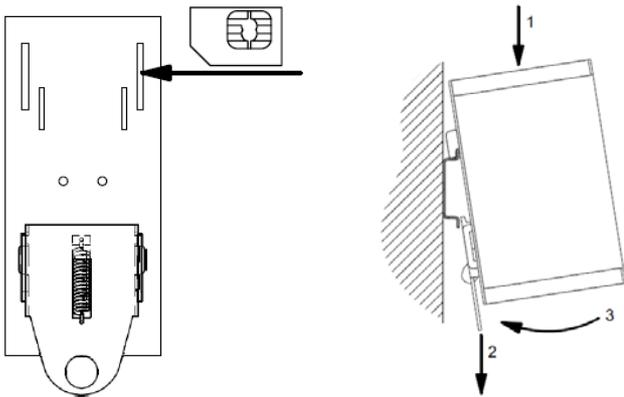
Insert the SIM card in the device's rear before the installation on the DIN rail. The device must be switched off.
